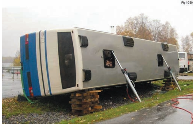
Plate 18.16. If people are trapped under a bus constructed of steel, it can be quickly lifted with extended hydraulic cylinders in the corners of roof hatches or with two air bags.
