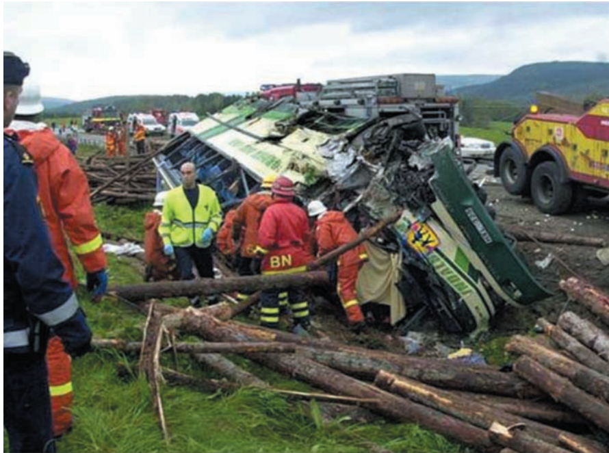
Plate 18.13. A timber truck with trailer suffered a front tire blow out and became so difficult to steer that it crashed into an oncoming school bus in rural, northern Sweden in 2001. Timber entered the bus and made the rescue effort extremely difficult. Six of the 42 passengers involved died. Used with permission from Scanpix.
