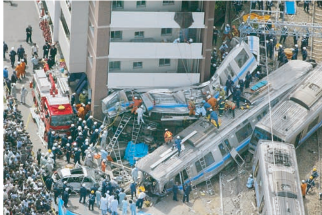
Plate 18.11. A Japan Railway express train derailed in 2005, and jackknifed against a parking garage in an urban area of Amagasaki, Japan. The crash left 107 passengers dead and injured 549. Used with permission from Scanpix.
