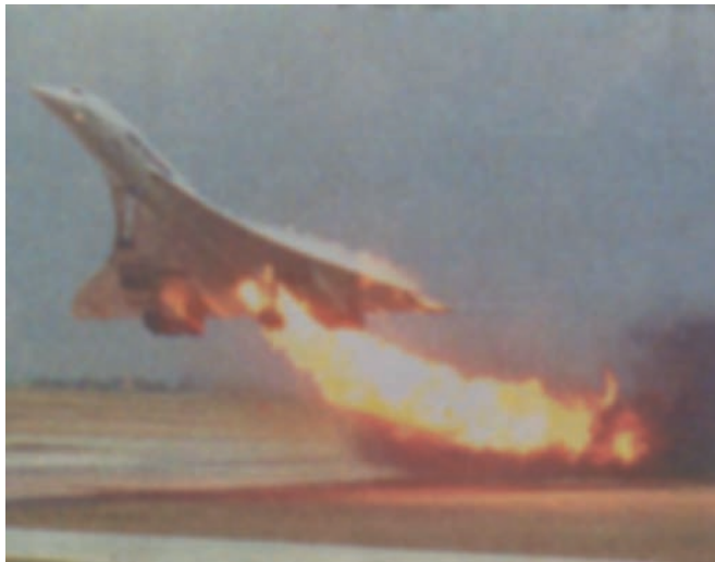
Plate 18.2. The Concorde's last flight in the year 2000. A piece of metal on the runway caused a tire explosion. Debris from the tire punctured the wing fuel tank and the fuel caught fire. Photo from Associated Press. Available at: http://www.airdisaster.com/photos/afsst/2.shtml .
