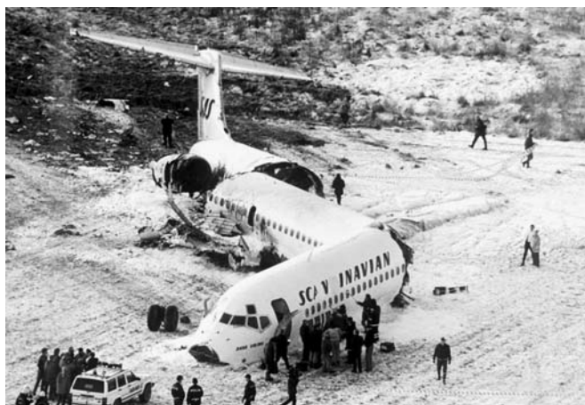
Figure 18.3. The 1991 MD-81 crash in Stockholm was caused by engine failure at low altitude when clear ice from the wings was sucked into the engines. During the emergency landing, the aircraft's momentum was reduced by hitting a number of trees before crashing on a snowy field. The snow probably prevented a postcrash fire. See color plate.
