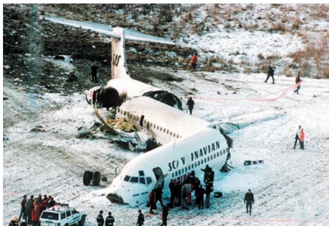
Plate 18.3. The 1991 MD-81 crash in Stockholm was caused by engine failure at low altitude when clear ice from the wings was sucked into the engines. During the emergency landing, the aircraft's momentum was reduced by hitting a number of trees before crashing on a snowy field. The snow probably prevented a postcrash fire.
