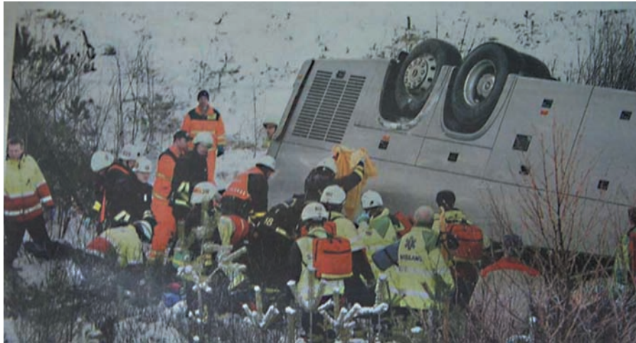
Plate 18.14. This tour bus drove off the highway and down an embankment, hit a boulder, rolled 180°, and landed on a roof that subsequently collapsed. Nine passengers died, but only two had lethal injuries. Six were jammed between the roof and interior structures (usually a seat back), and suffocated due to immobilization of the chest. It took 3.5 hours to extricate the surviving passengers.
