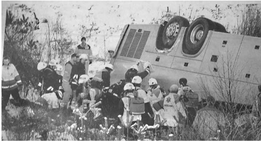
Figure 18.14. This tour bus drove off the highway and down an embankment, hit a boulder, rolled 180°, and landed on a roof that subsequently collapsed. Nine passengers died, but only two had lethal injuries. Six were jammed between the roof and interior structures (usually a seat back), and suffocated due to immobilization of the chest. It took 3.5 hours to extricate the surviving passengers. See color plate.
