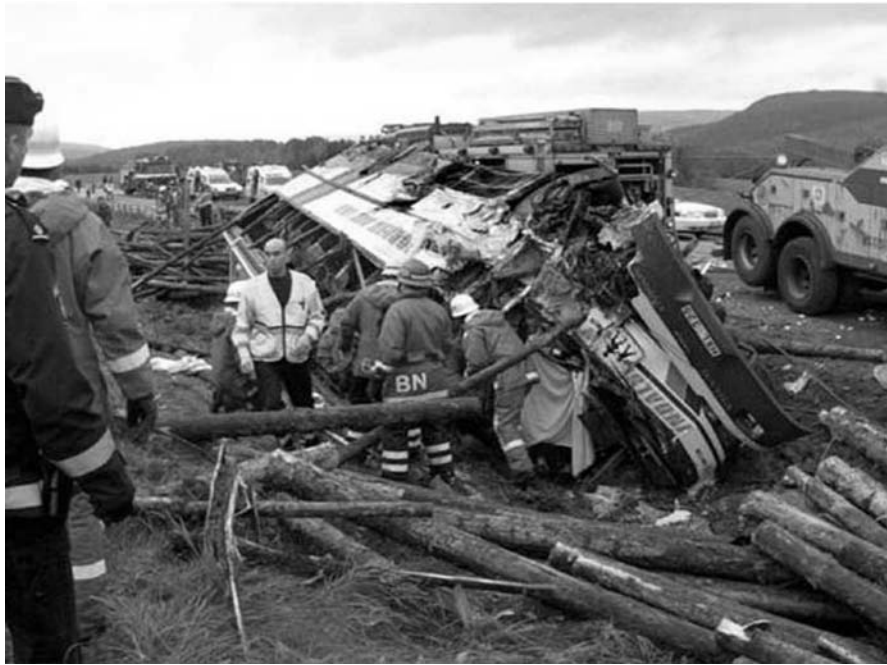
Figure 18.13. A timber truck with trailer suffered a front tire blow out and became so difficult to steer that it crashed into an oncoming school bus in rural, northern Sweden in 2001. Timber entered the bus and made the rescue effort extremely difficult. Six of the 42 passengers involved died. See color plate. Used with permission from Scapix.
